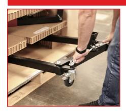
Remove parts from shipping crate in the order directed. Lock wheels on base (J) to provide stability.
