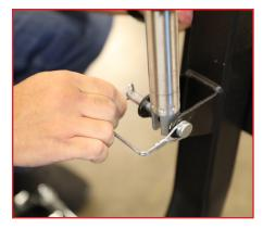
Attach actuator #1 (F) to the bracket on base arm (C) and secure clevis pin. Slowly lower boom arm (B) until it rests in the air on its own, making sure that it is supported by actuator #1 (F).
