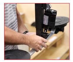
Attach cup assembly (E) to boom arm (B) by sliding metal into the opening and secure clevis pin located on actuator #4 (L).
