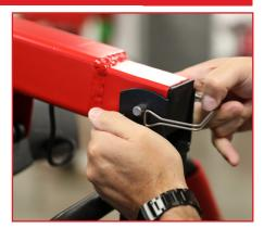
Using two people, lift boom arm (B) and align with top of base arm (C). Secure clevis pin.
