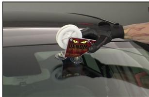
Continue to insert the wire from the Venom™ under the moulding all the way around the windshield until you are where the wire was inserted through the urethane.
