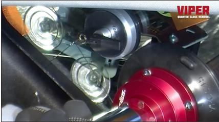
Towards the end of the removal, the mini anchor may move slightly due to the torque being produced by the Viper™ - this is normal.
