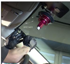
Once the clip/setting pin is cut, you can then continue cutting across the top of the windshield. Be sure to take special care not to get hungup on the wiring harness for the rearview mirror.
