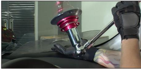
As you make your way around the windshield, you will have to reposition the Viper™ unit as needed for the proper cutting angle.
