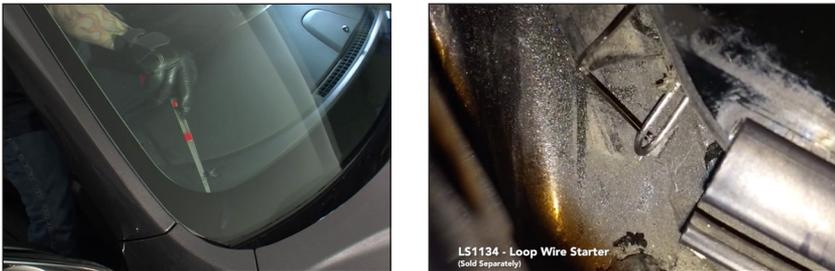
Note: To avoid damages to the painted area it is recommended to place a piece of tape on the exterior of the pinchweld.
