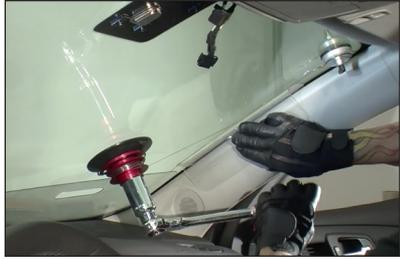
Continue cutting down the A-pillar until the wires cross making the final cut and the wire simply reels back into the vehicle. The removal is complete. You can now remove the mini anchor and Viper™ unit and proceed to lift out the windshield and prep for replacement.
