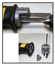
Remove base mounting screw (#2652L) (x1) with HOP 3/16 Hex Bit
