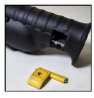
Pull the blade release lever forward to dislodge and remove from assembly
