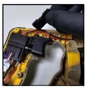
**9**Remove lock latch from top of switch
