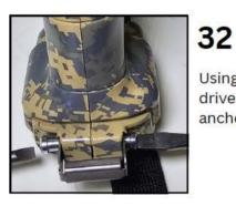
Using 2 flat head bits (1 screw driver / 1 drill) to tighten anchor bolt
