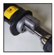
Remove base mounting screws (#2652s) (x2) with HOP 5/32 Hex Bit
