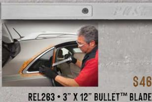
Bullet™ Blades are elongated, rounded blades designed to cut from all angles. Their unique shape and sharpening make side-to-side cutting easier and make slicing through wide beads of urethane a breeze.
