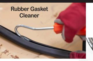
An easy way to get the grit, grime, old butal and shards of broken glass out of the tight spaces of a rubber gasket.
