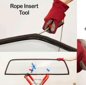
Insert the rope flawlessly into the gasket groove. Set the glass and secure it by dethreading the rope for speed and efficiency on your classic installation.
